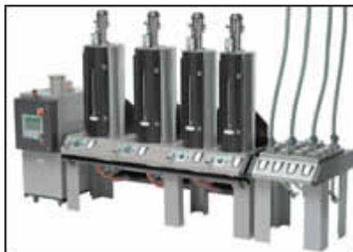
ResinWorks from Conair is a highly flexible, customizable new system of multiple drying hoppers on a single "sled." It permits quick material changes and precise control of individual hoppers.
