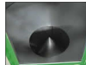
Solid-cone hoppers are easier to clean than perforated cones. (Photo: Foremost)
