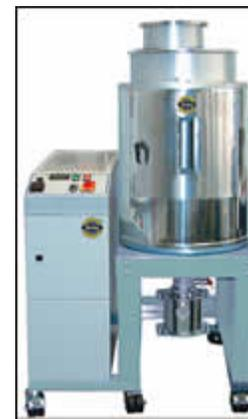
Some new compact units like Sterling’s STT40 have dryer sections resembling a small mold-temperature controller.
