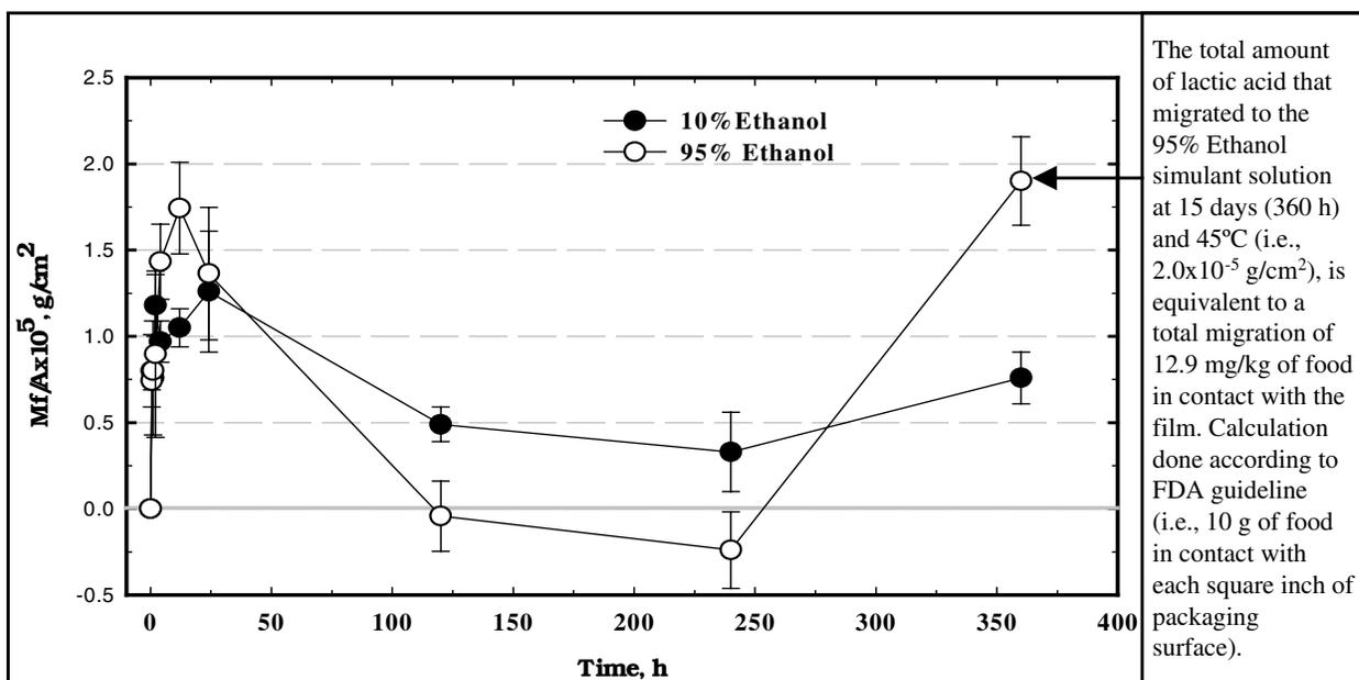
**Figure 8.** Mass migrated into the food per unit of area of polymer in  $\text{g/cm}^2$  versus time. Simulant solutions 10% Ethanol and 95% Ethanol. The gray line indicates the zero baseline.
