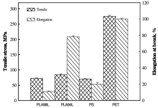
Figure 3. Tensile stress and Elongation at break of PLA98L, PLA94L, PS and PET
