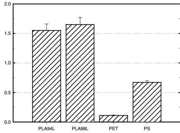
Figure 5. Water Vapor Permeability Coefficients of PLA94L, PLA98L, PS and PET at 30°C and 100%RH
