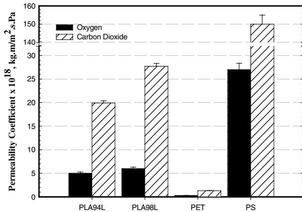
Figure 4. Oxygen and Carbon Dioxide Permeability Coefficients of PLA94L, PLA98L, PS and PET at 25°C and 0% RH.
