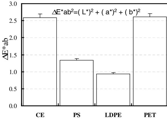
Figure 2.  $\Delta E^*ab$  values for PLA, CE, PS, LDPE, PET, and CE films.  $L^*$  is the lightness, and  $a^*$  and  $b^*$  the radii of chromaticity.
