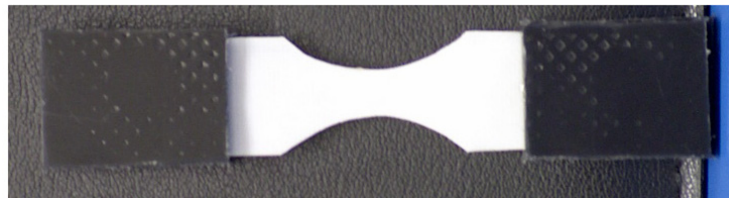
Figure 3: Tensile specimen with nylon stubs on both ends.
