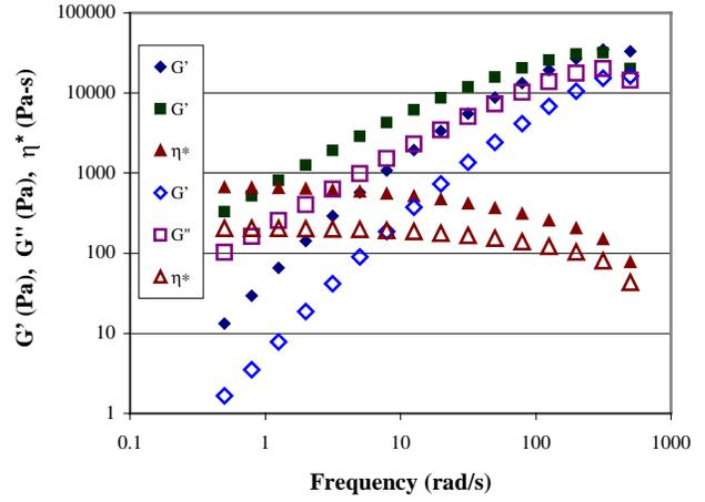
**Fig. 2.** Dynamic rheology properties for Polypropylene. Filled symbols are  $T = 180^\circ\text{C}$  and blank symbols are  $T = 210^\circ\text{C}$ .
