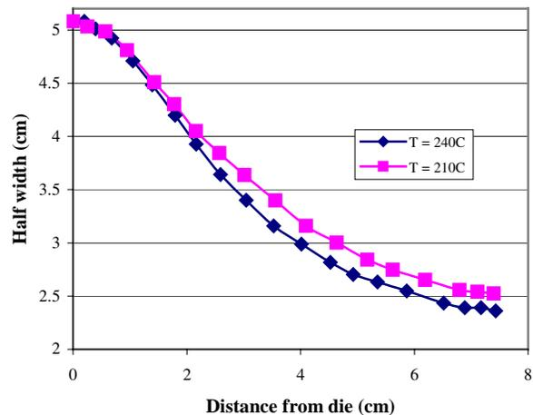
**Fig. 6.** Width profile for PP as function of die temperature.
