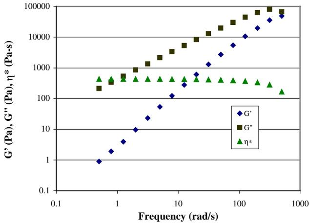
**Fig. 3.** Dynamic rheology properties for Polyethylene terephthalate at  $270^\circ\text{C}$ .
