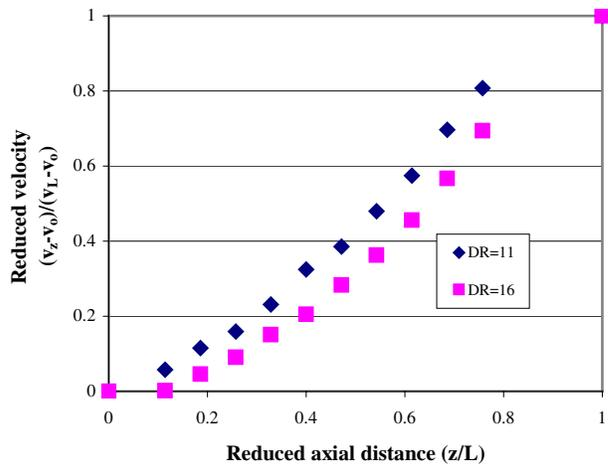
**Fig. 8.** Centerline velocity profile for PP as a function of draw ratio.
