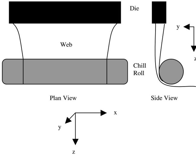
**Fig. 1.** Film casting Schematic
