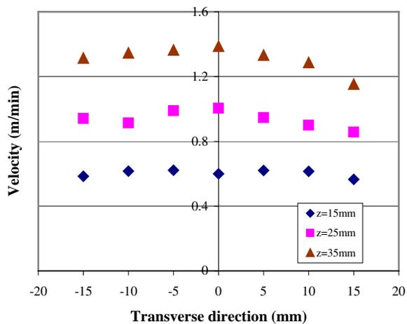
**Fig. 7.** Transverse direction velocity profile for PP.
