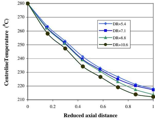
**Fig. 4.** Centerline temperature profile for PET.
