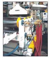
Luigi Bandera's new corotating twin-screw extruder with patented venting recycles PET bottle flake into film without drying or crystallizing.
