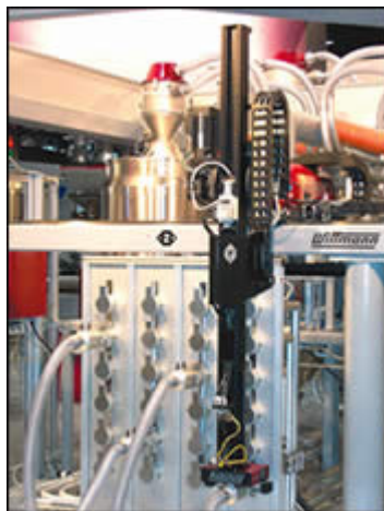
Wittmann's new Robofold automated material-distribution manifold uses a robot to switch material lines.
